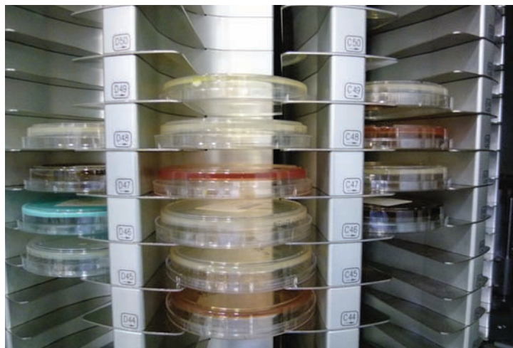
WASPLab Incubator; image courtesy of COPAN Diagnostics.
