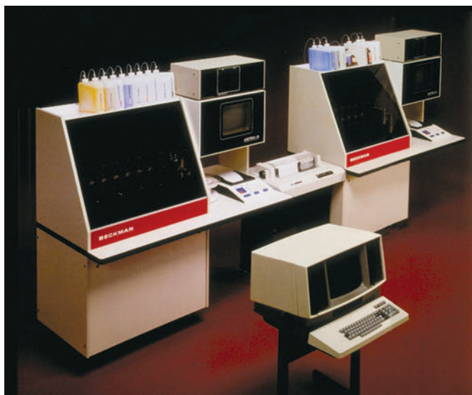
Figure 1. ASTRA 8 (Automated Stat Routine Analyzer) – 1978. Microprocessor controlled chemistry analyzer capable of measuring sodium, potassium, chloride, CO 2 , glucose, blood urea nitrogen, and creatinine in one minute.
