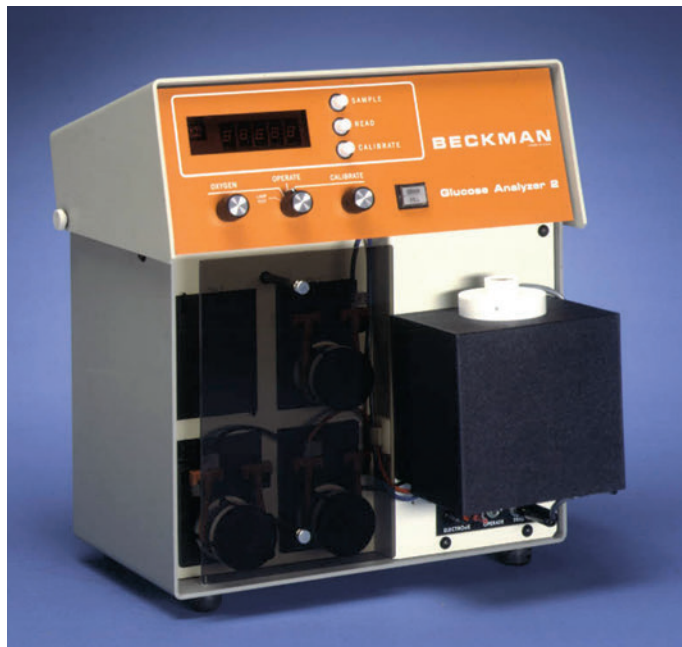
Figure 3. Glucose Analyzer 2 – 1979. Single channel benchtop analyzer measuring glucose levels in serum, plasma, and urine samples using an glucose oxidase electrode.
