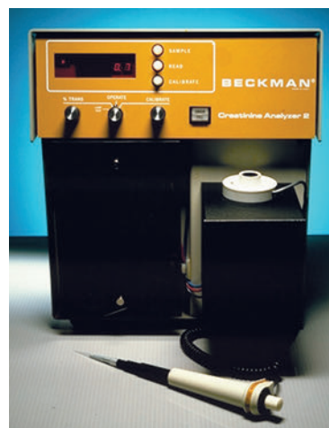
Figure 2. Creatinine Analyzer 2 – 1979. Single channel benchtop analyzer measuring creatinine levels in serum, plasma, and urine samples using an enzymatic Jaffe reaction.
